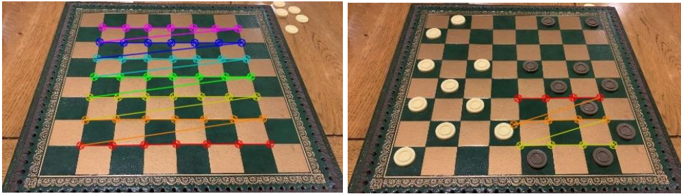
Figure 15 - findChessboardCorners() function with (7x7) filter (left) | findChessboardCorners() method with 3x4 filter(right)
